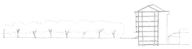
Figure 12. CS7, Technical Engineering School, Bejar; the environment analyse and assessment is important for the consideration of building physics and energy of this building. There could be no doubt that sun orientation and shading curtain wall facing west is a part of the concept of this recent heritage construction. Simulation of light and airflow can be provided from studies of section and dynamic flow.
