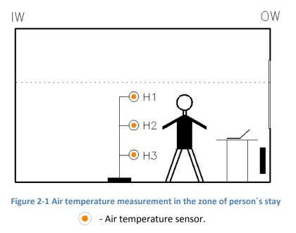
For a long-time monitoring it is possible to install the temperature sensor at the height H2 near indoor walls (Figure 2-2), in the case when preliminary measurements show, that the air temperature doesn't change a lot over the room depth. It is necessary to remember that this temperature represents only general tendency of the temperature in the room.
