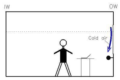
Figure 2-7 Air velocity measurement with unidirectional/bidirectional anemometers under the window
