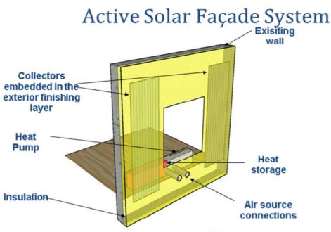
Over the test period - from Jan 2012 to May 2012.-global measured system COP for the heating mode was 3.78 for the active façade system and 2.87 for the reference system (air only heat pump)
