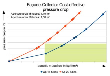
Picture 5: Pressure drop curve of the new Cost-Effective air collector
