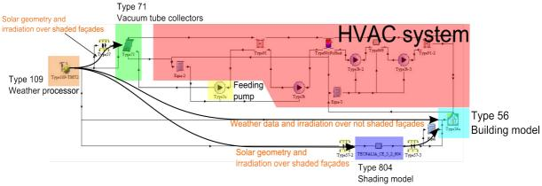
Picture 9: Model of a vacuum tube solar air collector for both HVAC and shading performance analysis **vertical plane**
