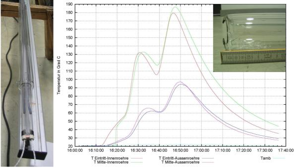
Picture 11: Researches according to the fracture behaviour of glass tubes depending on thermal friction
