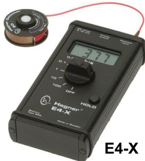
Figure 22. The Hagner E4-X illuminance meter is equipped with a V-lambda filter for adaption of the human eye and a cosine filter to compensate for the incidence.
