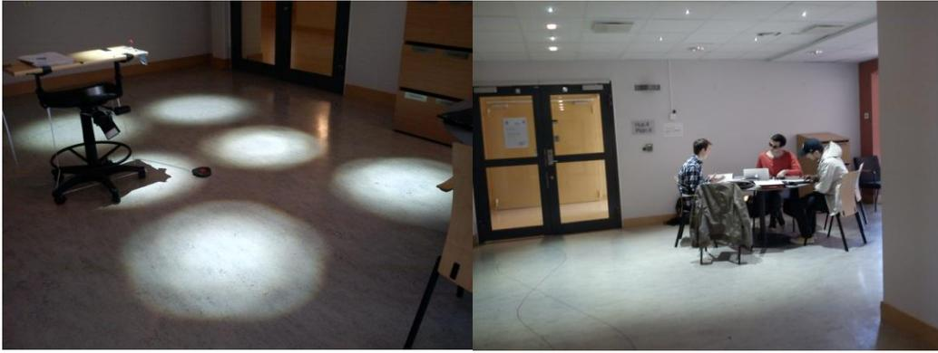
Figure 31. The output light distribution obtained from the L3 spot luminaires (left) and directly from the fiber ends (right). The table seen in the left picture was used for illuminance measurements at the test site at 85 cm above the floor.
