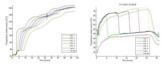
Figure 13: Measured temperature profiles in the zeolite reactor (TR1-TR5) and temperature of the air inlet and outlet during charging (left) and discharging (right) of the system.
