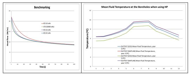
Figure 7: (left) Comparison between a simple implicit model (EES10) and analytical solutions and CFD data, (right) Comparison between the simplified model implemented in Matlab and the specific software EED (Earth Energy Designer)
