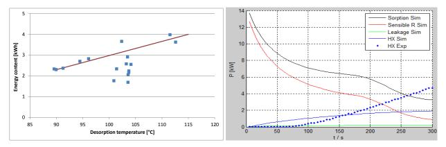
Figure 15: Energy content of the TNO 3 kWh reactor vs. desorption temperature (left) and model calculation (lines) and experimental values of thermal powers as a function of time (right) for a particular experiment.
