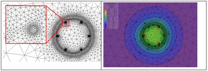
Figure 6: Calibrated high detail 3D-FEM models to analyse the performance of new materials in thermoactive foundations.
