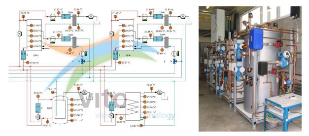
Figure 17: Schematic of the experimental setup with instrumentation and picture of the test rig in the lab.
