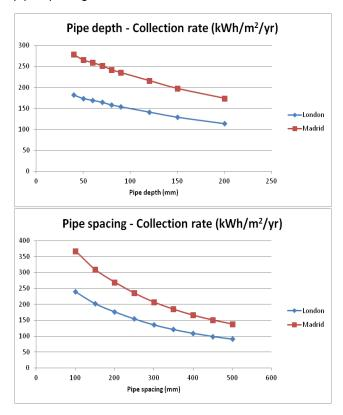
Figure 9: Annual heat collection curves of road solar collector as a function of pipe depth (left) and pipe spacing (right) in the climates of London and Madrid.
