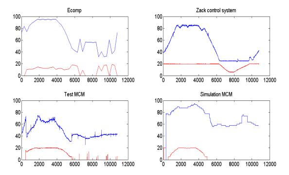
Figure 27: Results of the 4 runs **without** storage: blue line: output power of the mGT, red line: output power of the ICE
