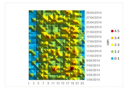
Figure 31: Three-dimensional representation of the electricity consumption of the 'Balk van Beel' in April 2014 in kWh per hour (kW)
