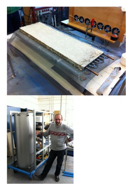
Figure 14: Heat exchanger (left) and reactor vessel containing eight heat exchangers (right).
