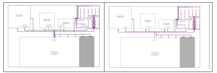
Figure 8: (left) first variant that uses a single heat pump room inside a centrally located building, from which high temperature thermal energy is distributed, (right) second variant that consists of two separate (but connected) networks over which low temperature is distributed for use by heat pumps inside the buildings.
