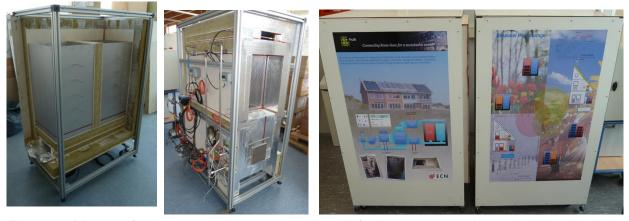
Figure 12: Pictures of the open sorption storage system. Left, the storage vessels, and middle the air handling unit both under construction. Right, the sorption system in its final state in the laboratory.
