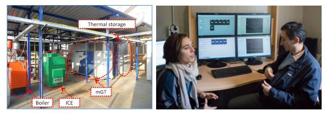
Figure 25: Left: equipment at the lab at TPG-DIME, with a boiler, an Internal Combustion Engine CHP (ICE), a micro gasturbine CHP (mGT) and thermal storage vessel. Right: TPG-DIME personnel at the data acquisition and control system.
