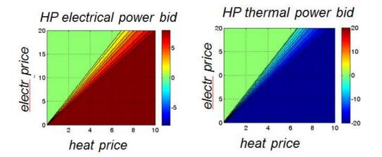
Figure 19: Electrical power bid surface (left) and thermal power bid surface (right) of a heat pump. The colours represent the amount of power the heat pump is willing to produce as a function of the prices of heat and electricity. As an example, at an electricity price of 5 €ct/kWh and a heat price of 6 €ct/kWh the heat pump will be fully on, consuming 6.7 kWh of electricity and producing 20 kWh of heat
