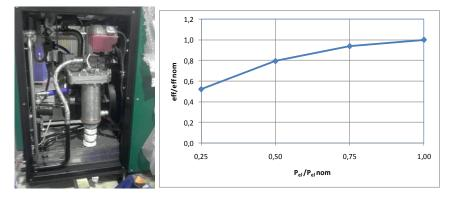
Figure 5: Picture and electrical efficiency an internal combustion engine CHP at partial load.
