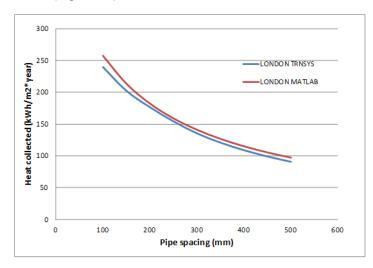
Figure 11: Annual heat collected by a typical layout of road solar collector, as function of pipe spacing, for the climates London. Comparison between results of simple Matlab model and TRNSYS
