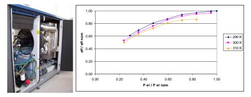
Figure 4: Picture and electrical efficiency of the micro gas turbine CHP at partial load for different ambient temperatures
