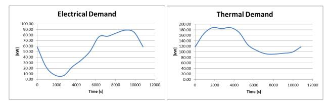
Figure 26: Conflicting profiles: low electrical demand and high thermal demand in the first half of the test and vice versa in the second half.
