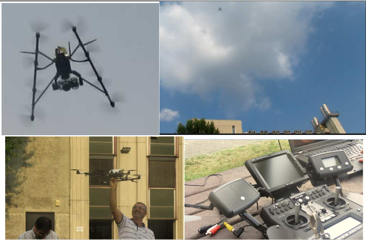
Figure 26: Falcon 8 UAV equipped with a FLIR Tau 640 camera and a HR RGB camera
