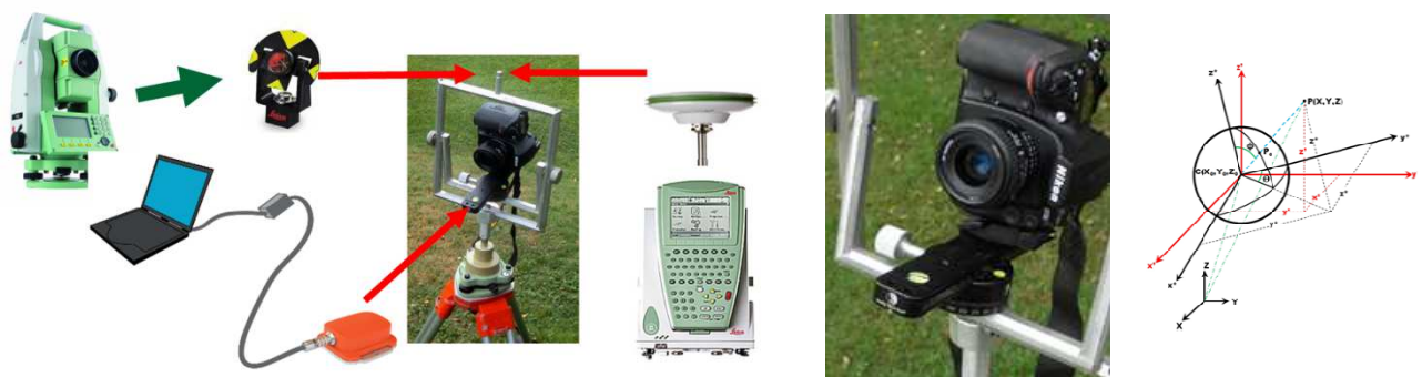
Figure 5: The panoramic head used to generate gnomonic images
