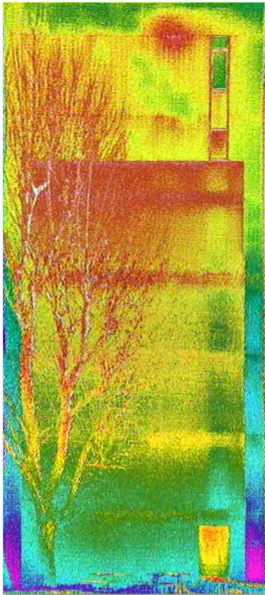
Figure 28: Facade thermal orthophoto: March 2013 (a), July 2013 (b)
