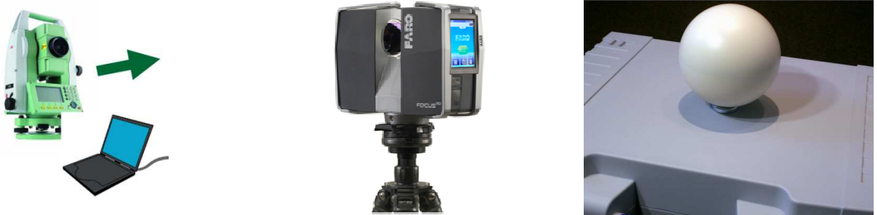
Figure 4: 3D TLS (Terrestrial Laser Scanning) for rapid detailed model acquisition of dense cloud points to be processed for both the simplified model and the detailed model
