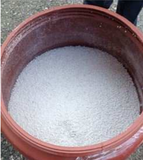
1 - Storage of the hydrophobic expanded perlite delivered by S&B.
