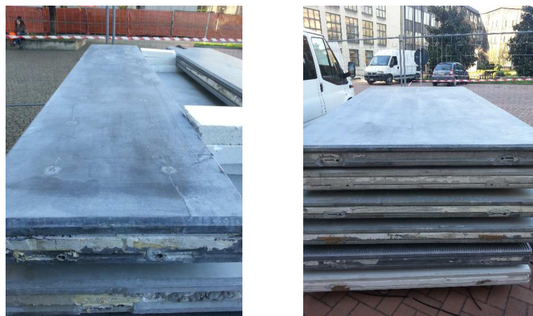
Figure 20: Panels before installation stored in the test facade site
