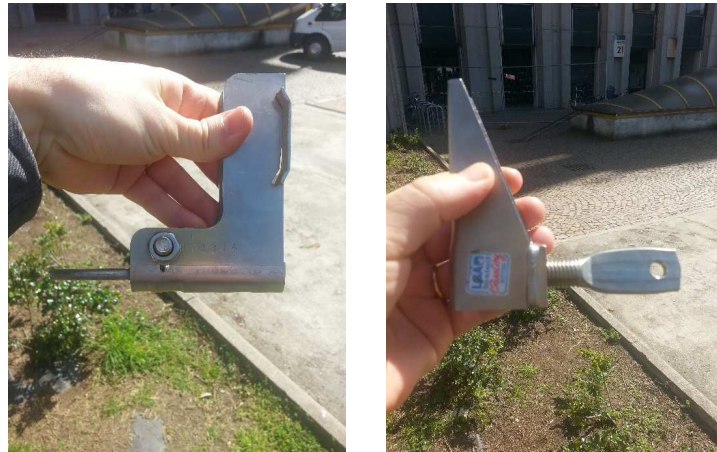
Figure 21: Halfen body anchor type DT. Right side Halfen body anchor type BA
