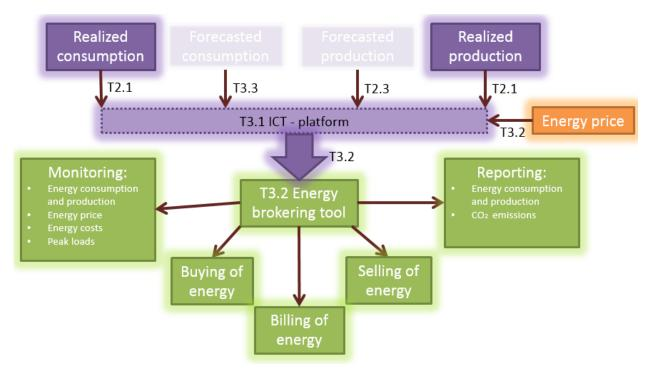
**Figure 4:** Energy Brokering Tool utilizes ICT-platform (interfaces and database) to connect to building automation and/or metering systems.
