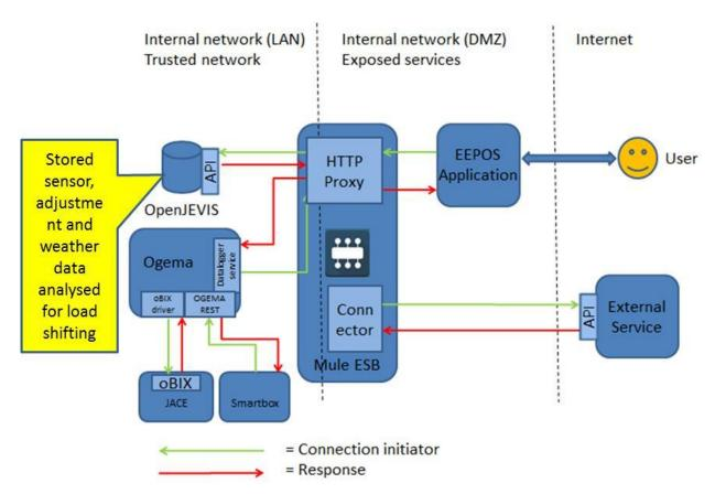
Figure 6: Automatic adjusting of software relation with system architecture defined in D3.1
