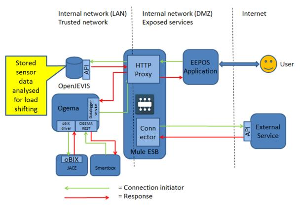
**Figure 7**: Automatic cut of high consumption relation with system architecture defined in D3.1
