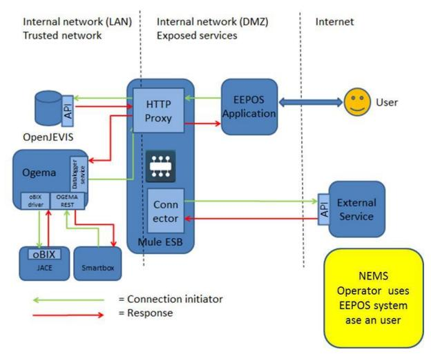
Figure 2: NEMs operator located in the EEPOS system architecture defined in D3.1
