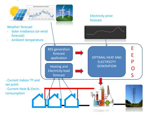
Figure 11: Power & Heat EEPOS system architecture
