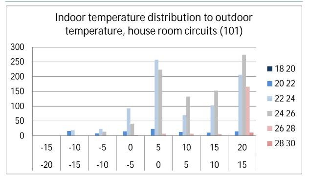
Room temperature remote control unit use per outdoor temperature
