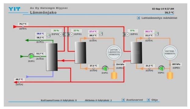
Figure 10 District heating process view for remote controlling
