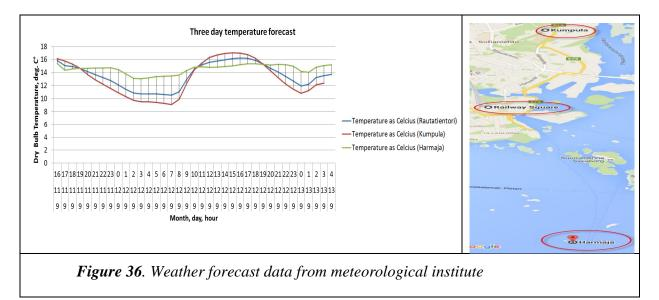
As an conclusion from the graph is that altough the distance from Kumpula weather station to Harmaja only 13 km the temperature forecast for each site varies by number of degrees. A second conclusion is that since the Merenkulkijanranta is onshore Harmaja weather station data should be more close to the weather data collected by WXT520. In this point was also noticed that most of Harmaja weather data is missing and that the demonstartion building do not have collection of full year data.
