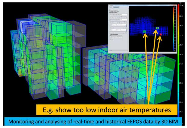
*Figure 20* Example of VTT's BimZone tool's BIM based visualizing and analysing: which spaces has too low indoor temperatures on selected time period – case Finnish demonstrator
