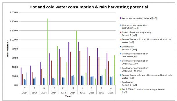
*Figure 35* Domestic hot and cold water consumption & rain water harvesting potential
