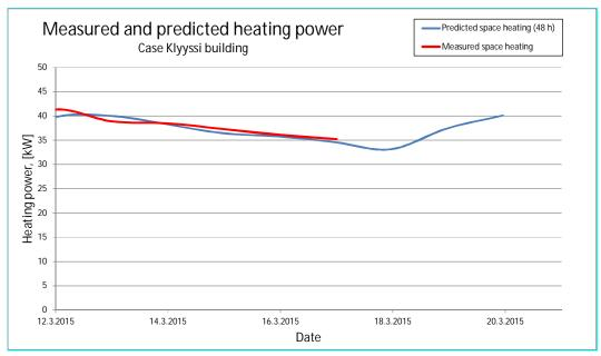
Figure 17 Space heating related energy consumption forecast – case Finnish demonstrator.
