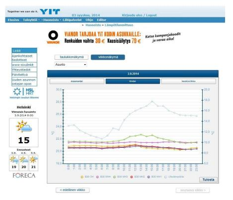
*Figure 13 Temperature view for resident. Highest line present outdoor temperature. Lower lines present room specific temperatures in household.*
