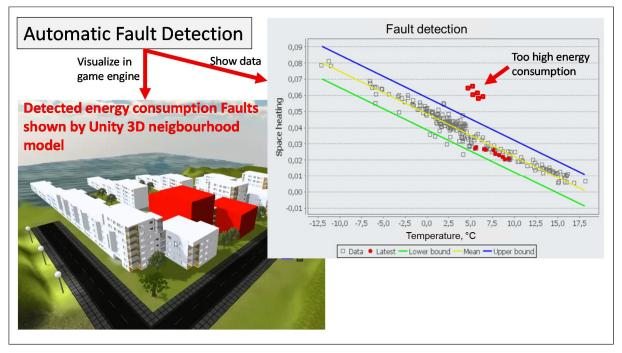
Figure 19 Space heating related fault detection – case Finnish demonstrator
