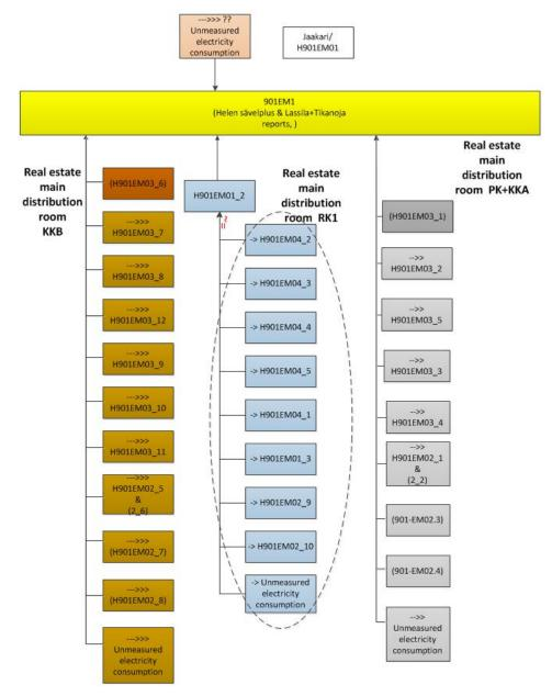
Figure 26 Hierarchical structure of electricity meters
