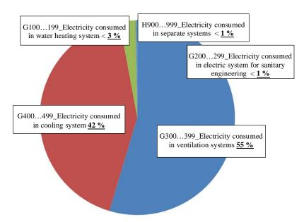
Figure 28 Electricity consumption, sampling width 26.6.2014 - 31.8.2014
