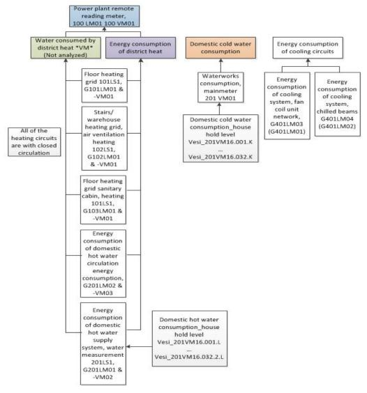
*Figure 27 Distributed heat, cool and hot water and cooling meters hierarchical structure*
