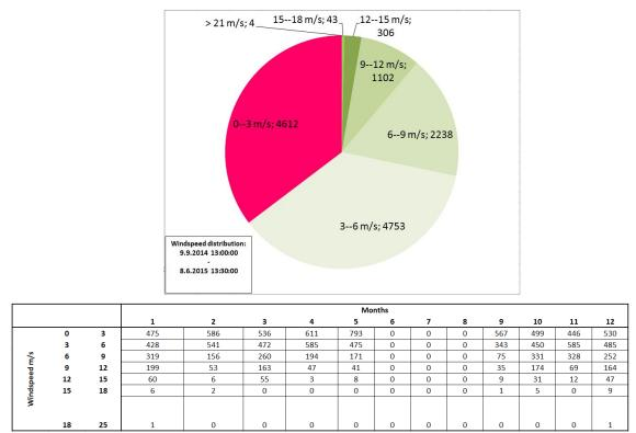
*Figure 41* Wind speed distribution by wind speed (top) and wind speed distribution by wind speed and month
