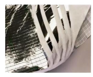
Figure 7 : Multi layers thermal insulation technology
