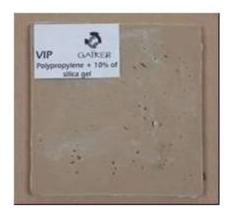
Figure 55. PP filled with fumed silica from VIP waste (Source: GAIKER)
