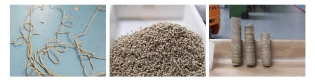
Figure 68. Extrusion products from multilayer films with aluminium (Source: GAIKER)
