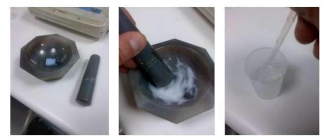
**Figure 49.** Sample preparation for viscosity measurement (first tests with aerogel sample coded ID 012 Pure TEOS)
