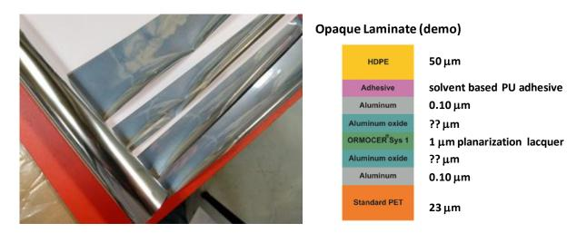
Figure 25. Details of different layers in the structure of the O-VIP envelope
