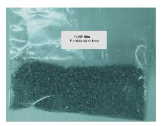
Figure 64. O-VIP film shredded for EoL options evaluation, particle size <1mm.
