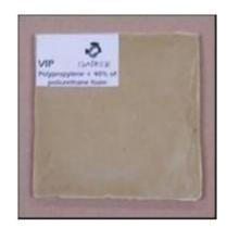
Figure 59. PP filled with PU foam from VIP waste (Source: GAIKER)
