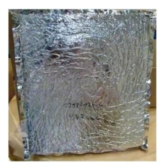
Figure 18. Sample of the O-VIP panel (BASF) received at GAIKER facilities.
