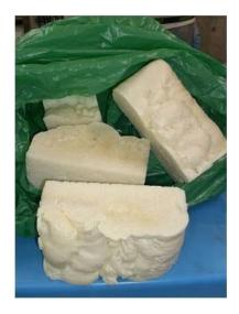
Figure 62. PU rigid foam used as feedstock for glycolysis evaluation
