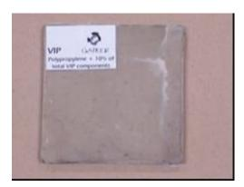
Figure 40. PP filled with silica VIP waste (Source: GAIKER)
