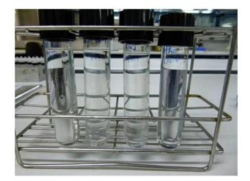
**Figure 67.** Chemical delamination tests by immersion of O-VIP and T-VIP laminate samples in acid and basic solvents at room temperature
