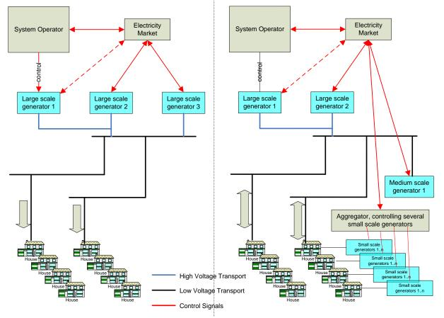
Figure 1. Traditional (left) vs. Smart transport & distribution grids
