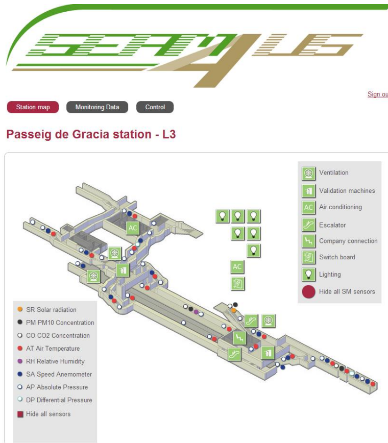
Figure 26. 'Station map' tab showing the position and values of all sensors
