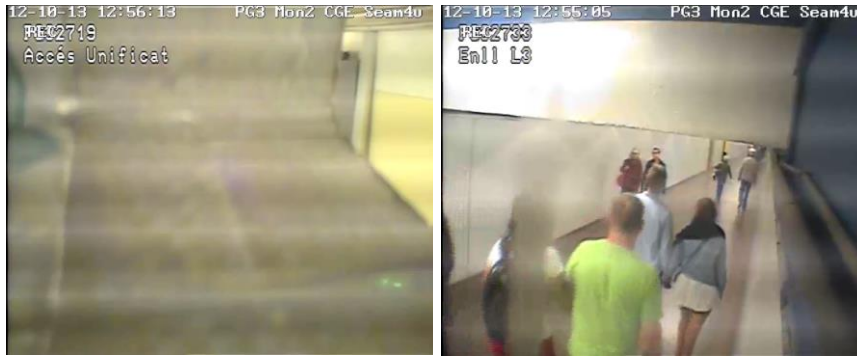
Figure 15. Examples of CCTV malfunctioning: (left) occluded camera; (right) scratched camera
