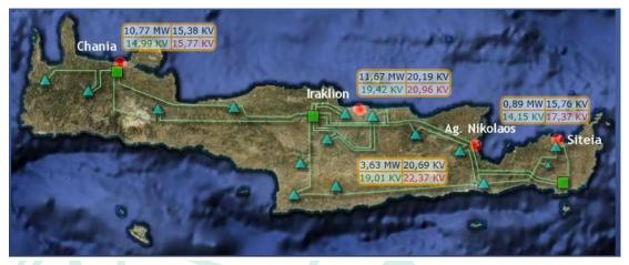
Figure 37 - Transmission Grid of Crete and optimal power flow visualization
