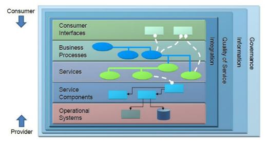
Figure 5 The Open Group SOA RA Logical Solution View (Source: The Open Group)
