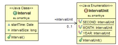
Figure 24 Globally used object for defining an interval
