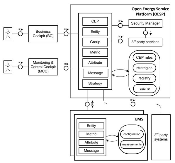
Figure 11 SmartKYE Service Architecture
