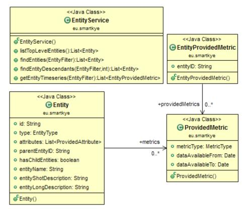
Figure 12 The Entity Service of the platform
