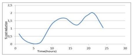
Figure 40 Cost reduction as a function of the time of wash for cost curve B and wash energy of 1kWh
