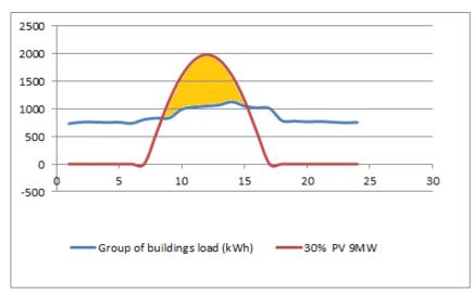
Figure 49 Energy curtailment for a group of buildings with PV installed capacity of 9MW
