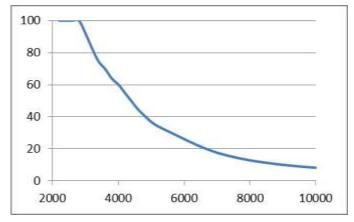
Figure 65 Curtailment reduction as a function of installed PV capacity for wash energy of 4kWh and 120 washing machines
