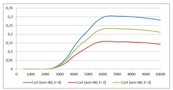
Figure 73 Reduction in PV investment payback time for feed-in tariff=0.25e/kWh and cost=0.1euros/kWh (120 washing machines)
