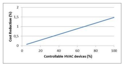
Figure 78 Consumer cost reduction as a function of controllable HVAC for price curve A
