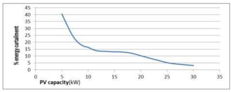
Figure 28 Reduction in Curtailment for low temperatures.
