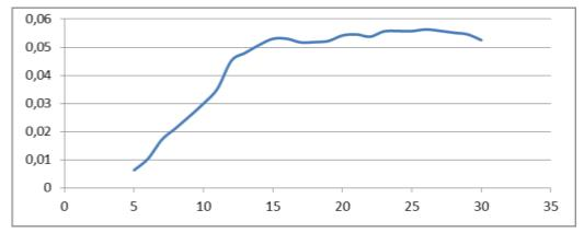
Figure 37 Reduction in PV investment payback time for feed-in tariff=0.25e/kWh and cost=0.1euros/kWh
