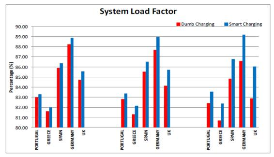
Figure 9 The increase of system load factor comparing "dumb charging" with "smart charging" (Home charging- winter)
