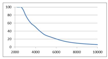
Figure 67 Curtailment reduction as a function of installed PV capacity for wash energy of 3kWh and 120 washing machines
