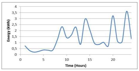
Figure 14 load curve of a small building
