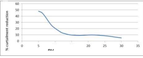
Figure 29 Reduction in Curtailment for high temperatures.
