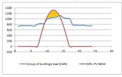
Figure 46 Energy curtailment for a group of buildings with PV installed capacity of 6MW
