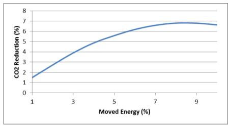
Figure 87 CO2 emissions reduction (%) as a function of the total energy moved (%) for 174 MW of installed wind power
