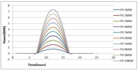
Figure 44 Typical PV production for 1-10MW photovoltaic generators.
