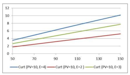
Figure 71 Curtailment reduction as a function of the number of washing machines for wash energy of 2-4kWh and installed PV capacity 10 MW.
