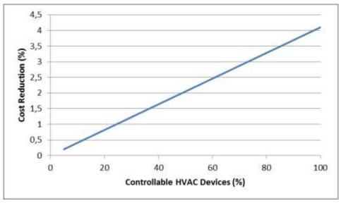
Figure 79 Consumer cost reduction as a function of controllable HVAC for price curve B
