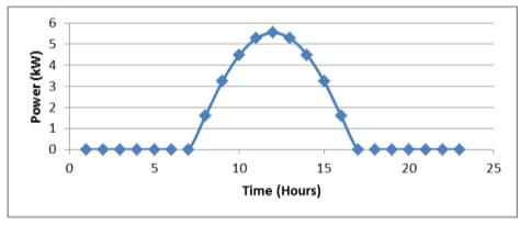
Figure 25 Typical PV production for a 10kW photovoltaic generator
