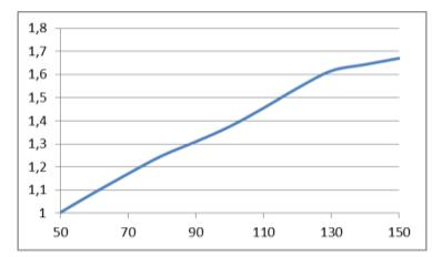
Figure 56 PV curtailment reduction as a function of the number of HVAC devices for installed PV capacity of 10 MW
