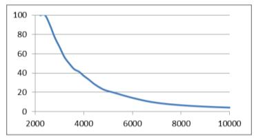
Figure 66 Curtailment reduction as a function of installed PV capacity for wash energy of 3kWh and 80 washing machines
