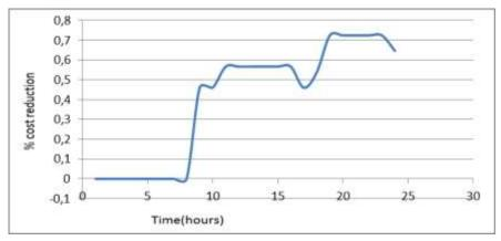
Figure 39 Cost reduction as a function of the time of wash for cost curve A and wash energy of 0.5kWh
