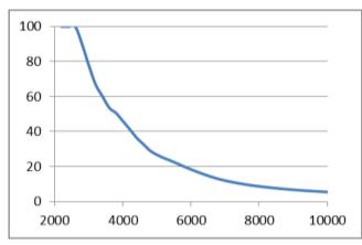
Figure 64 Curtailment reduction as a function of installed PV capacity for wash energy of 4kWh and 80 washing machines
