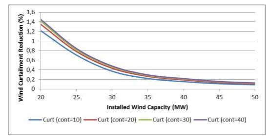
Figure 76 Wind curtailment reduction as a function of the installed Wind capacity (MW) for various levels of controllable HVAC
