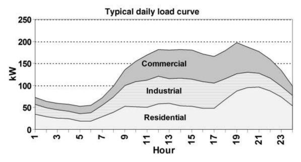
Figure 5 Typical load curve for each feeder of the study case network
