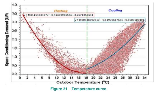
The curve of temperature of 2012 is used for the controllable HVAC loads.
