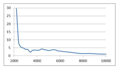
Figure 59 PV curtailment reduction as a function of the installed PV capacity 50 HVAC devices and cold year
