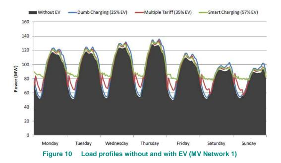
**Changes in the load diagrams**: The extra power demanded by EV provokes several changes in the networks' load diagrams, which are more pronounced as the EV integration
