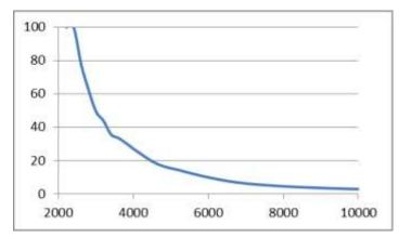
Figure 68 Curtailment reduction as a function of installed PV capacity for wash energy of 2kWh and 80 washing machines
