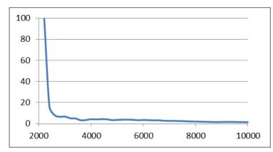
Figure 57 PV curtailment reduction as a function of the installed PV capacity 100 HVAC devices and cold year
