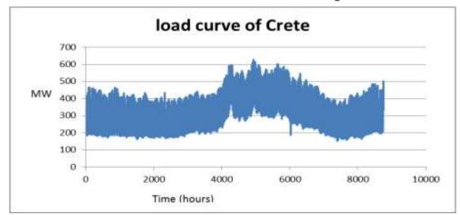
The load curve of Crete of 2012 is used for the load curve of large communities.
