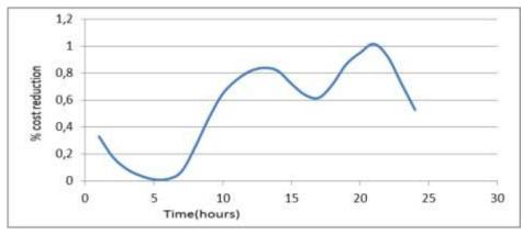
Figure 41 Cost reduction as a function of the time of wash for cost curve B and wash energy of 0.5kWh
