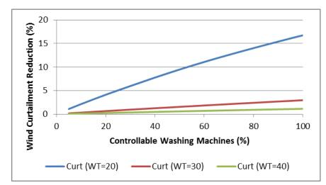
Figure 81 Wind curtailment reduction as a function of controllable washing Machines for various levels of installed Wind capacity (MW)
