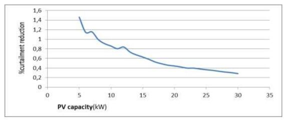
Figure 36 Reduction in Curtailment if initial washing hour is 20.00 and wash energy 0.5kWh
