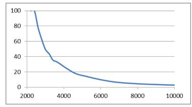
Figure 69 Curtailment reduction as a function of installed PV capacity for wash energy of 2kWh and 120 washing machines
