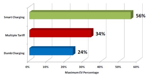
Figure 7 Maximum EV integration percentage in the MV Network 1
