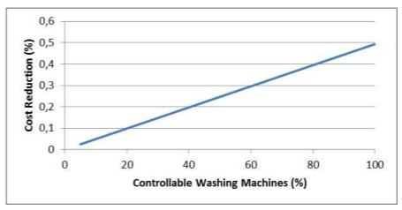
Figure 83 Consumer cost reduction as a function of controllable Washing Machines for price curve B
