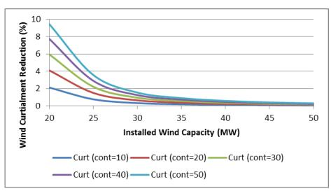
Figure 80 Wind curtailment reduction as a function of the installed Wind capacity (MW) for various levels of controllable Washing Machines
