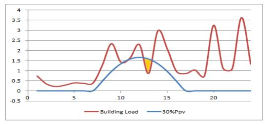
Figure 27 Energy curtailment for a building with PV installed capacity of 10kW.
