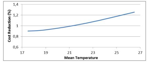
Figure 31 Cost reduction as a function of mean temperature for Cost Curve A
