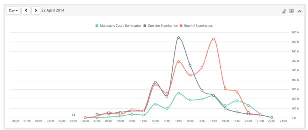
Figure 63 - EMTE light level measurement at Room 1, Multisport Court and Corridor
