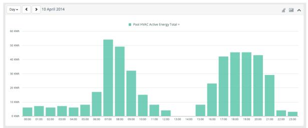
Figure 50 - EMTE swimming pool HVAC thermal consumption
