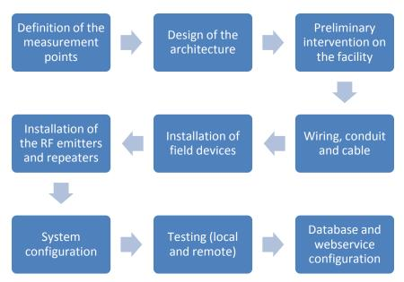
Figure 4: Installation procedure of the How Module
