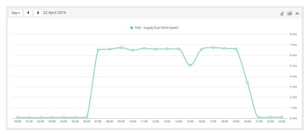
Figure 62 - FIDIA pilot HVAC duct air speed
