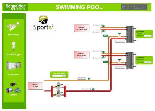
Figure 5: Swimming pool water heat exchanger system graphics.
