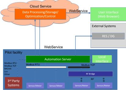
Figure 2: HOW Module Architecture
