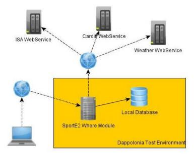
Figure 7: Deployment diagram
