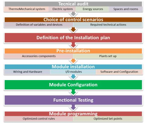
Figure 3: Installation sequence of the WHEN Module.
