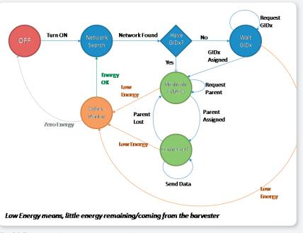
Fig. 20: Transitions between operation modes.
