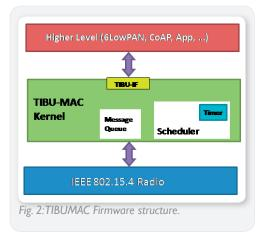
The structure of the TIBUMAC firmware is shown in Fig. 2. The gateway is constantly powered and its available energy is supposed to be infinite. On the other hand, the functional behaviour of the nodes may change depending on their available resources.
